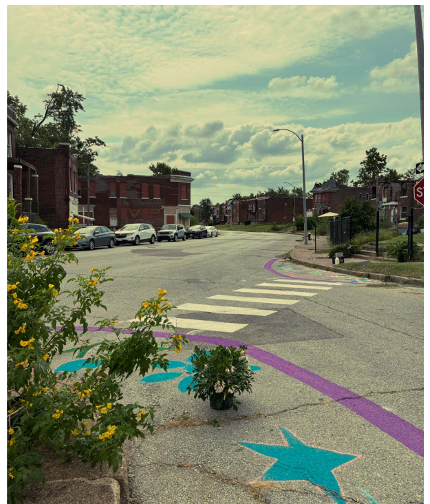
Above: A Trailnet traffic calming pop-up in Area 1 (August 2025), demonstrating how temporary street design interventions, such as paint and modular materials, can reduce speeds and improve safety for all road users.
